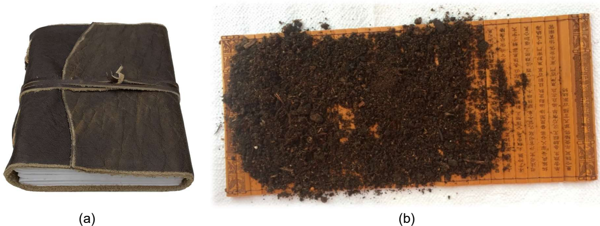
Fig. 2: (a) Exemplary self-made book consisting of 56 handmade paper pages, writings of different inks and a buffalo leather cover. The dimension of the book is approx. 17 cm \times 13 cm \times 3 cm (length \times width \times height). This book was used for the Computed Tomography experiments. (b) Bamboo scroll covered in potting soil. The scroll was completely soiled, rolled up, and put in a plastic bag for measurements with the imaging modality.
